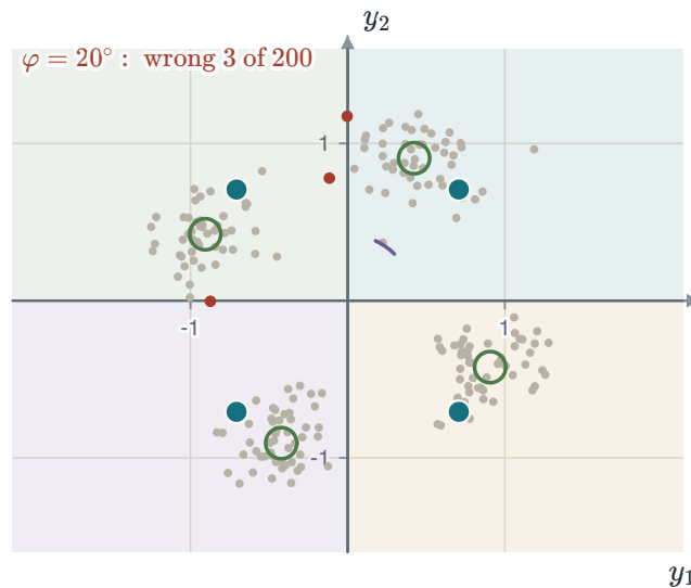
FIGURE 5.14 QPSK with 200 noisy symbols at a carrier phase error \varphi = 20^\circ , decided in the fixed quadrants. The green rings are the points turned by \varphi . Red dots are wrong decisions.
